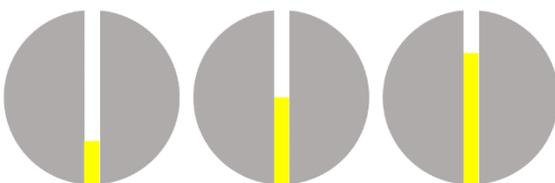
**Fig. 1.** Representation of the manual healing with MMA or PU of cylindrical specimens for 25 %, 50 % or 75 % of the crack length.
