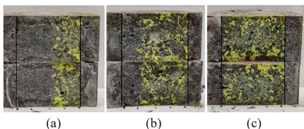
**Fig. 9.** Visual inspection of the manual crack healing with PU for (a) 25 %; (b) 50 %; (c) 75 % of the crack length.
