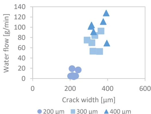
**Fig. 5.** Water flow as a function of the crack width for cylindrical specimens.
