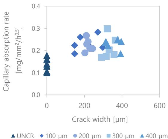
**Fig. 4.** Capillary absorption rate as a function of the crack width for cylindrical specimens.
