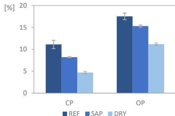
**Fig. 3.** Capillary porosity (CP) and open porosity (OP) for REF, SAP and DRY.
