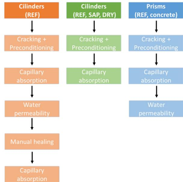
**Fig. 2.** Schematic overview of the testing program.
