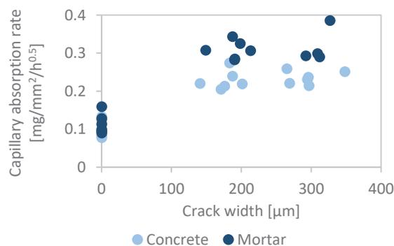
**Fig. 11.** Capillary absorption rate of prismatic mortar and concrete specimens as a function the crack width.
