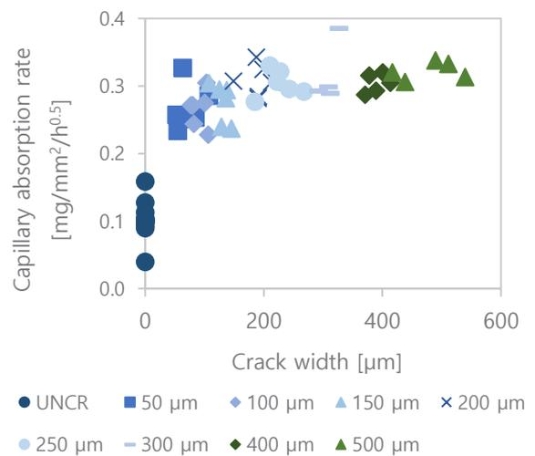
**Fig. 6.** Capillary absorption rate as a function of the crack width for prismatic specimens.
