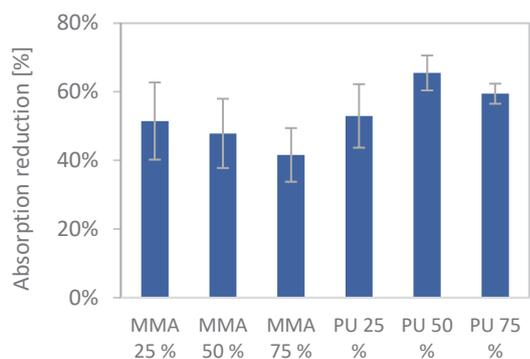
**Fig. 8.** Reduction of the capillary absorption rate of cylindrical specimens with silicon sheets with a nominal thickness of 200  $\mu\text{m}$  before and after healing with MMA and PU.
