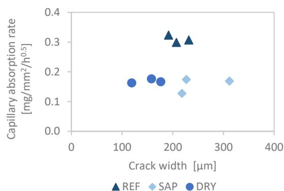
**Fig. 10.** Capillary absorption rate of prismatic specimens of REF, SAP and DRY as a function the crack width.
