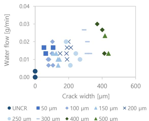
**Fig. 7.** Water flow as a function of the crack width for prismatic specimens.
