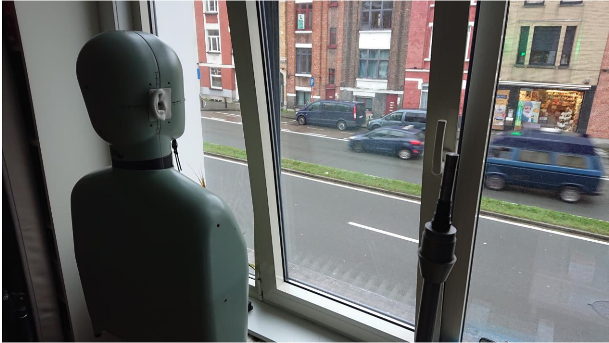
144 145 Figure 2. Photograph of the head-and-torso simulator, measuring binaural road traffic sound, 146 forming the basis for the sound reproduction in the virtual reality experiment. A frontal 147 positioning was chosen in front of a half-opened window in a real-life setting. 148
