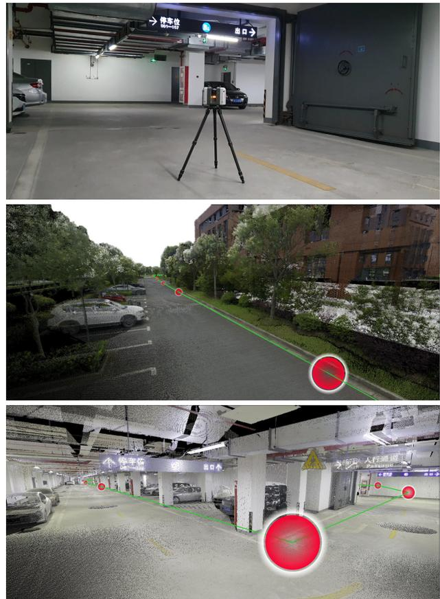
Fig. 8. Map construction by registering numerous individual scans as a whole with graph optimization.
