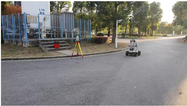
Fig. 11. Validation of the proposed mapping-localization ground truth system by a Leica MS60 (1mm accuracy) Laser Tracker.
