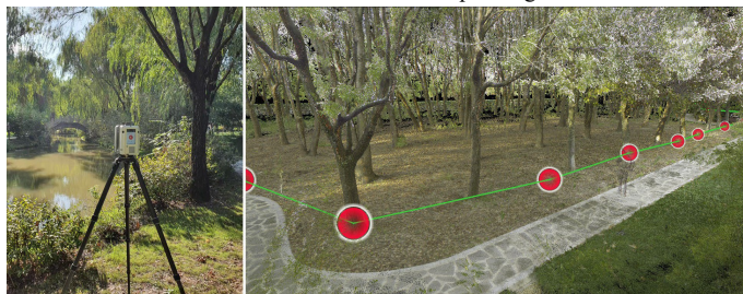
Fig. 6. Left: The surveying process. Right: The point cloud registration process.
