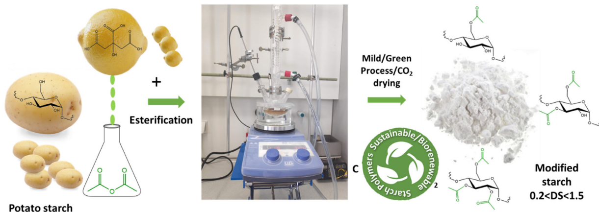
SCHEME 1 Schematic representation of the organocatalytic pathway for potato starch esterification coupled with supercritical CO 2 drying. Intermediate degrees of substitution ( 0.2 < DS < 1.5 ) [Color figure can be viewed at wileyonlinelibrary.com ]
