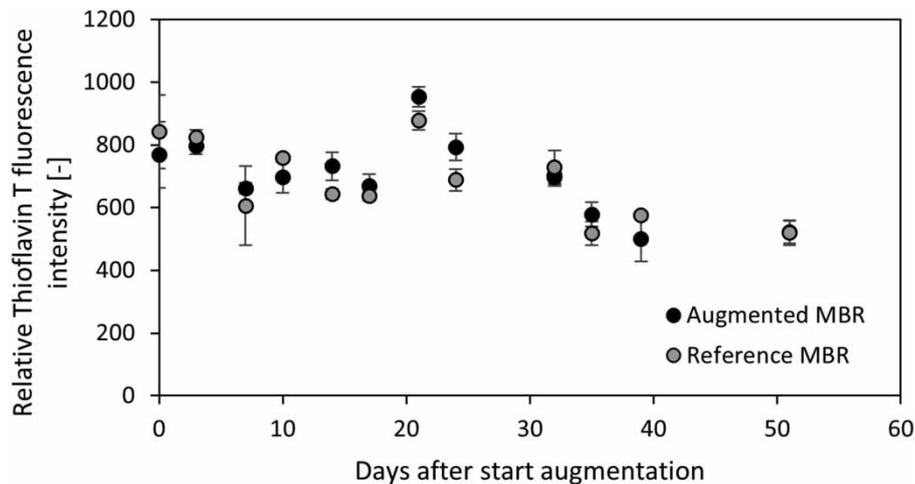
**Figure 12** | Evolution of ThT fluorescence intensity at  $490\ \text{nm}$  in the bioaugmented and reference MBR. Sample stained with  $10\ \mu\text{M}$  ThT relative to unstained sample. Each value represents the average of four technical replicates.
