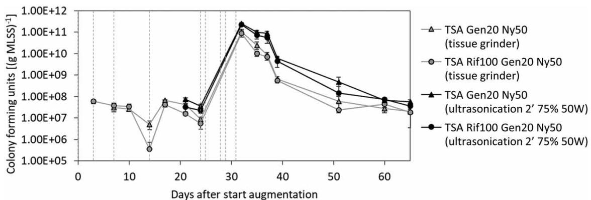
**Figure 9** | Evolution of colony-forming units in the augmented MBR. Deflocculated samples were grown on tryptic soy agar plates containing 20 mg L<sup>-1</sup> gentamycin, 100 mg L<sup>-1</sup> rifampicin, and 50 mg L<sup>-1</sup> nystatin selective for *Azoarcus communis* Rif<sup>r</sup>-mSc. Dashed lines indicate the bioaugmentation events. Analyses were performed prior to augmentation on the same day. Each value represents the average of six technical replicates.
