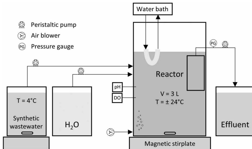
**Figure 2** | Schematic representation of the laboratory-scale MBR setup.
