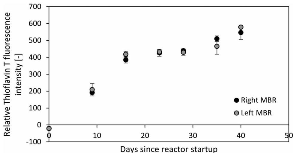
**Figure 7** | Evolution of ThT fluorescence intensity at 490 nm in the MBRs. Sample stained with 3- $\mu$ M ThT relative to unstained sample. Each value represents the average of four technical replicates.
