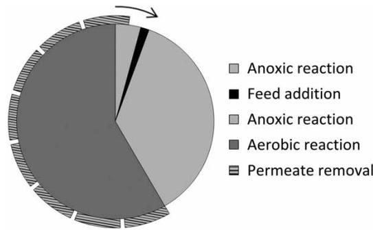
**Figure 3** | Schematic representation of the operational cycles of the laboratory-scale MBR setup. Total cycle time: 144 min.
