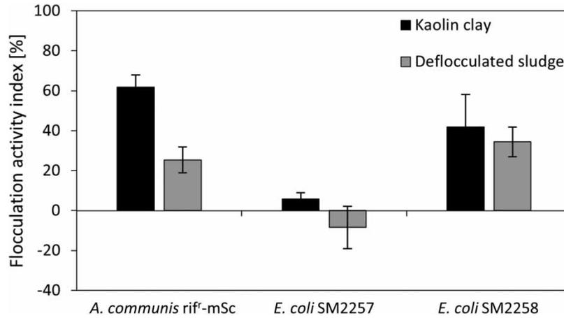
**Figure 6** | Flocculation activity against kaolin clay suspension and deflocculated activated sludge. After inoculation at an initial  $OD_{600}$  of 0.05, *Azoarcus communis* Rif<sup>r</sup>-mSc was grown in tryptic soy broth for 16.5 h, and the *Escherichia coli* SM2257 curli-deficient mutant and SM2258 mutant with upregulated curli production were grown in M63 broth for 48 h. Each value represents the average of three biological replicates. Error bars represent standard deviations.
