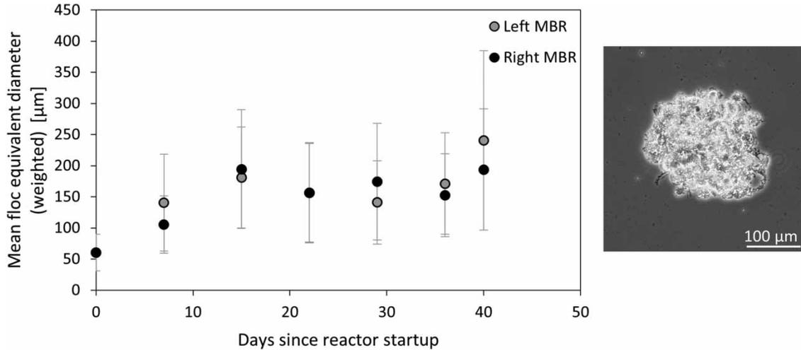
**Figure 8** | Sludge morphology. Evolution of the average equivalent floc diameter in the MBRs (left). Error bars represent standard deviations. Activated sludge floc with representative morphology taken from the left MBR at day 40 in phase contrast (right).
