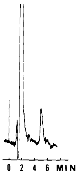
Fig. 3. HPLC recording of the fraction collected from the silica system and rechromatographed on the RP 8 column eluted with acetonitrile-water-acetic acid 79.6:20:0.4 (v/v) at a flow rate of 20 ml/hr, detection at 350 nm, and sensitivity at 0.005 AUFS. The retention time of the "unknown" corresponded to the retention time of all- trans -retinoic acid standard.
