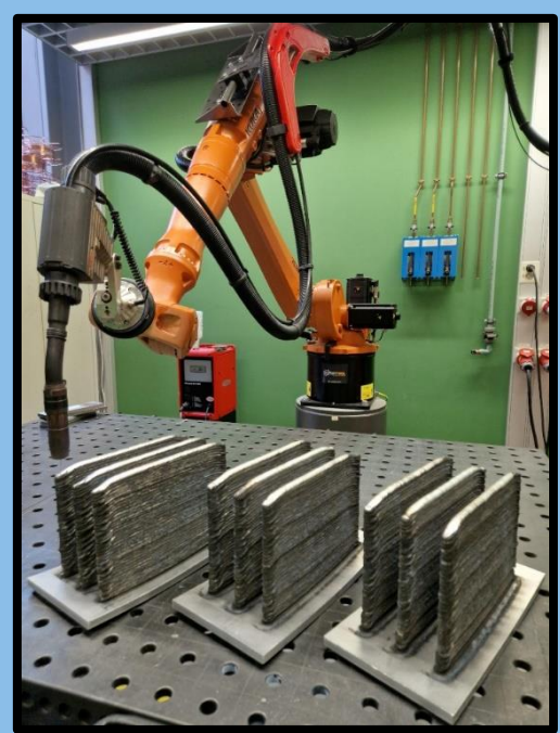
WAAM manufacturing of aluminium plates (image courtesy: BIL)
