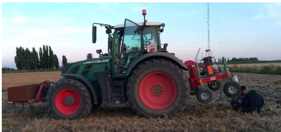
Figure 4. On-The-Go multisensory soil-sensing platform from Precision Soil and Crop Engineering group at Ghent University. This platform includes visible and near-infrared, gamma-ray, depth, and electrochemical sensors, as well as an RTK-GPS system among other devices.
