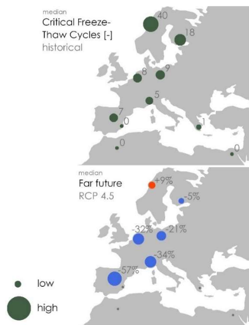
Figure 4. The median change in critical freeze-thaw cycles is generally decreasing. (Figure modified from [16]).
