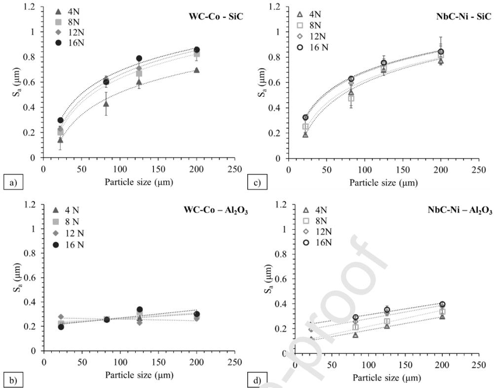
Fig. 9. Abrasive particle size vs 3D roughness of WC-Co against (a) SiC (b)  $Al_2O_3$  and NbC-Ni cermet against (c) SiC (d)  $Al_2O_3$  abrasives (Pristine  $S_a = 0.1 \pm 0.02 \mu m$ ).
