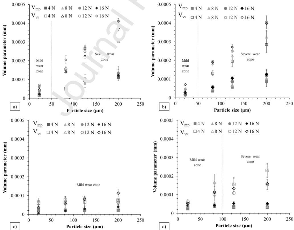
Fig. 10. Peak material ( $V_{mp}$ ) and valley void volume ( $V_{vv}$ ) of (a) WC-Co - SiC (b) WC-Co -  $Al_2O_3$  and (c) NbC-Ni - SiC (d) NbC-Ni -  $Al_2O_3$  cermet for different abrasive particle sizes.
