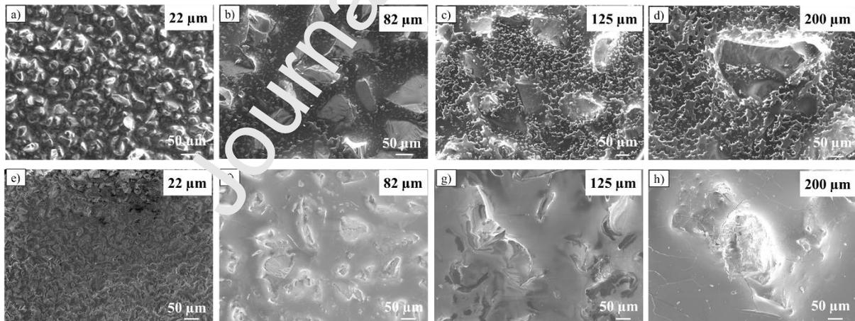
Fig. 3. SEM images of pristine SiC (a-d) and  $\text{Al}_2\text{O}_3$  (e-h) abrasives with different particle sizes from 22  $\mu\text{m}$  to 200  $\mu\text{m}$ .
