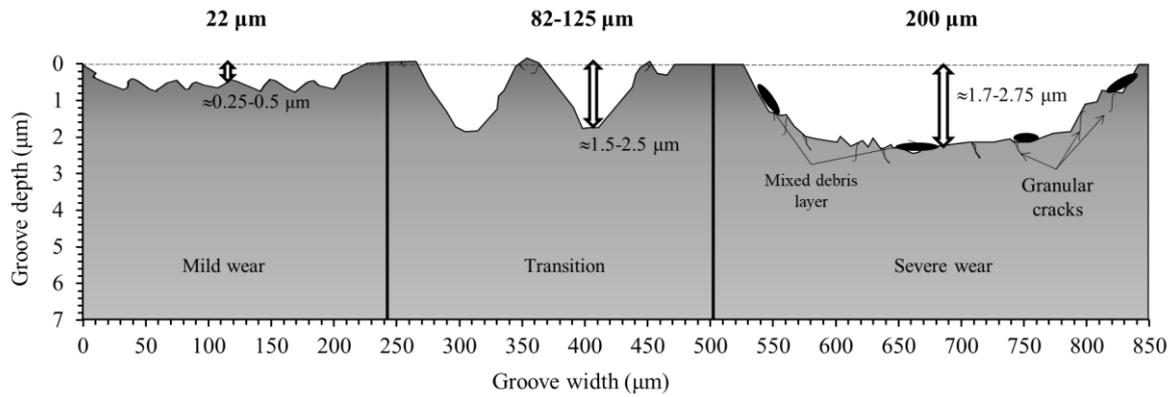
Fig. 11. Schematic cross-section of worn cermet surface as a function of SiC grit size.
