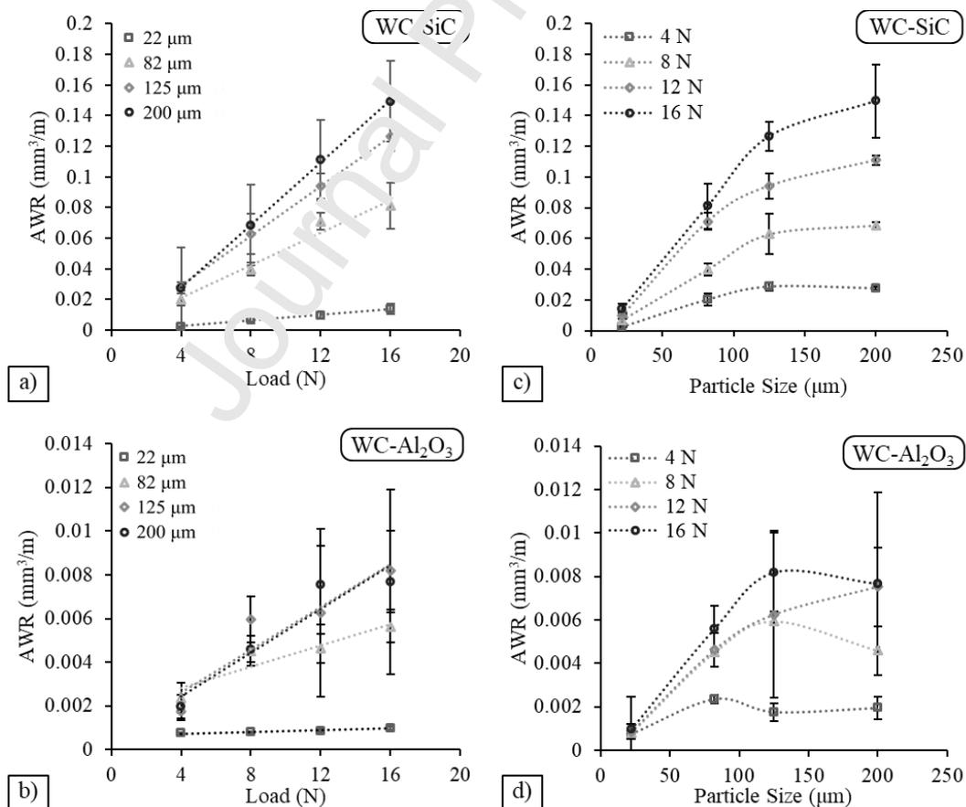
Fig. 5. Abrasive wear rate of WC-Co as a function of (a,b) load and (c,d) abrasive particle size for SiC (a,c) and Al<sub>2</sub>O<sub>3</sub> (b,d) abrasives.
