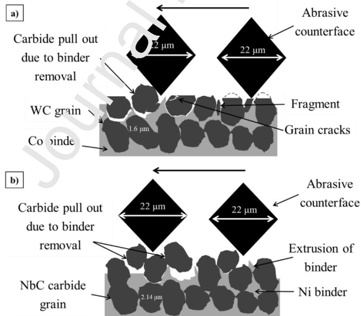
Fig. 15. Schematic wear mechanisms of (a) WC-Co and (b) NbC-Ni.
