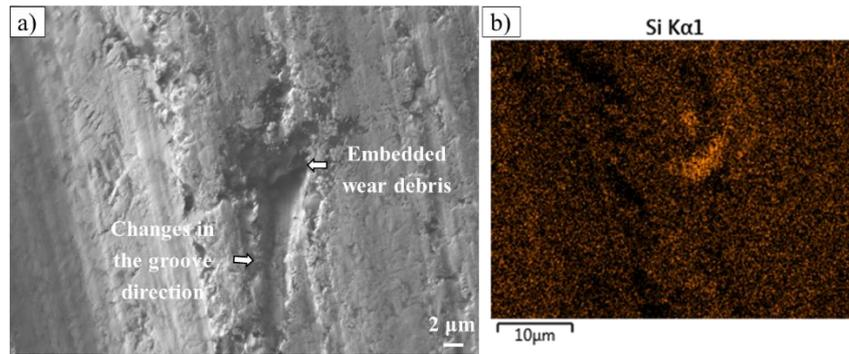
Fig. 17. (a) SEM micrographs of embedded SiC wear debris (b) EDS map confirms the presence of Si on the worn surface (Condition: WC-Co against SiC abrasive at 16 N load and 125  $\mu\text{m}$  abrasive size).
