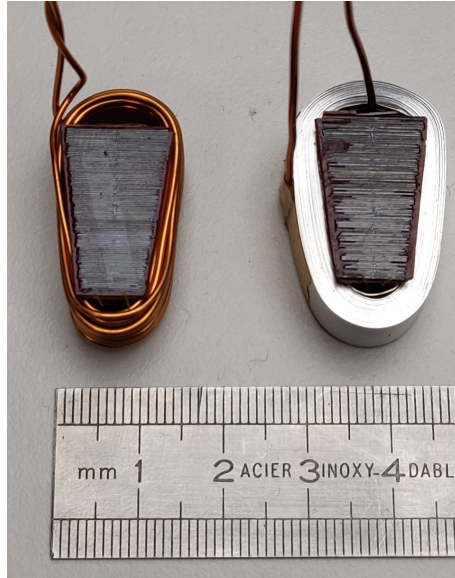
Figure 3.4: Prototype tooth coils: (left) enamelled copper wire (right) anodized aluminum foil
