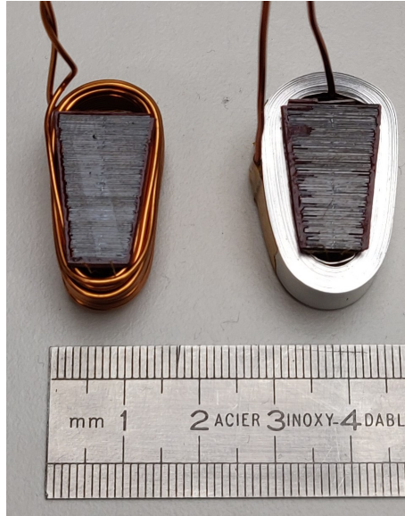
Figure 4.4: Prototype tooth coils. Left: enamelled copper wire tooth coil, Right: anodized aluminum foil tooth coil
