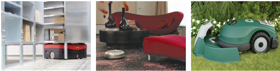
Figure 1.3: Well established applications of service robots: (a) Automated Guided Vehicles in warehouses [7] (b) vacuum cleaner robot [8] (c) lawn mower robot [8]
