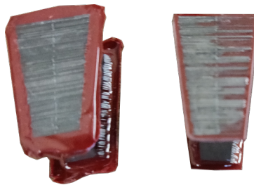
Figure 3.8: Epoxy potted stator tooth tips before (left) and after (right) mechanical grinding
