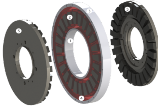
Figure 5.4: Yokeless and Segmented Armature Axial Flux Permanent Magnet Synchronous Machine: (1) Thermal end-winding interconnection ring (2) Concentrated winding tooth coil (3) Aluminum housing (4) Epoxy impregnation (5) Permanent magnet rotor.
