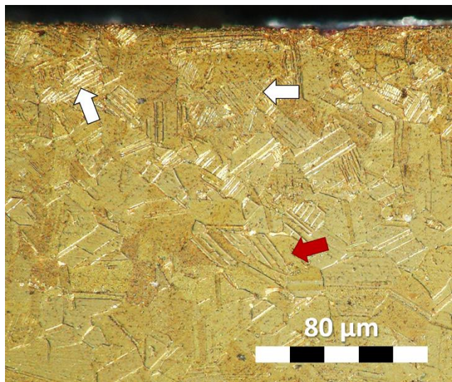
Fig. S7. Photomicrographs in polarized light of the transversal cross-section of one wire after metallographic etching. The main metallographic features are highlighted (red=twin lines; white=strain lines).
