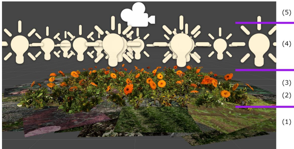
269 270 Figure 5: Simulation of a flower field in Unity to generate synthetic images. The 271 scene consists of different layers. From bottom to top: (1) background images of 272 weeds, (2) Calendula leaves, (3) Calendula flowers, (4) point lights, and (5) a 273 camera.
