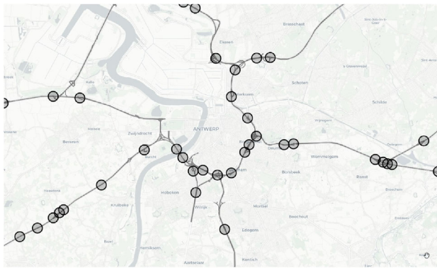
FIGURE 4 Static case investment: A subset of the fixed set of selected road-side unit locations ( I_{RSU} ), around Antwerp, Belgium.
