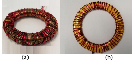
Fig. 12. Preparing the test sample with the measurement coils. (a) Fe-3Si, (b) Fe-6Si.
