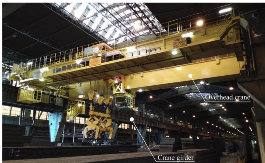
FIGURE 1: Principal components of an overhead crane assembly.
