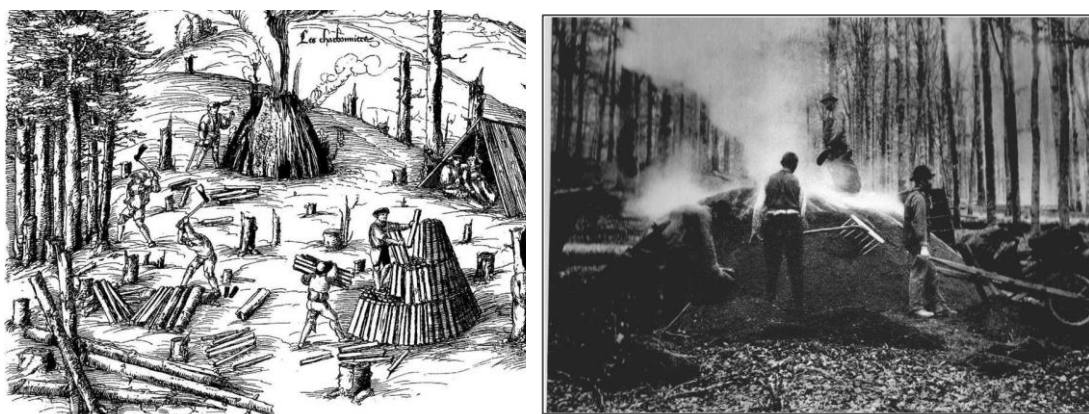
Figure B.1.3: (Left) Charcoal burning in 16 th century in France (Bert, 2007, Ludemann, 2010). (Right) Charcoal production in a mound kiln in the forest near Anlier, southern Belgium (Deforce et al., 2020).
