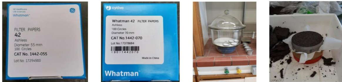
Figure 2. Whatman 42 filter papers, desiccator and container for filter paper samples
