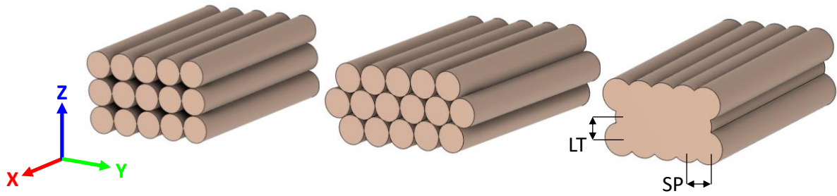
Figure 4 Schematic representation of possible printing strategies during printing of dense parts using 3D micro-extrusion: unidirectional stacking (left), unidirectional hexagonal stacking (centre) and unidirectional hexagonal stacking with overlap of the fibers and lower layer thickness that was adopted in this study (right).
