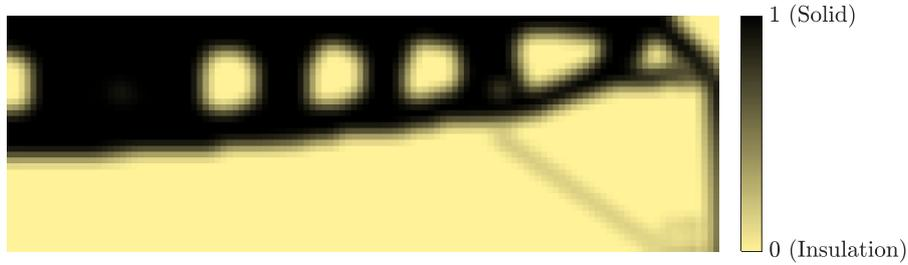
Figure 5: Optimized result for default parameter values:  $T_f = 800^\circ\text{C}$ ,  $F_m = 10\text{kN}$ ,  $t = 10\text{mm}$
