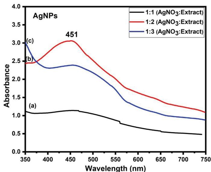
**FIGURE 4.** UV-Visible spectra of biosynthesized AgNPs from AgNO<sub>3</sub> to *Laggera* plant extract ratio of (a). 1:1, (b).1:2, and (c).1:3
