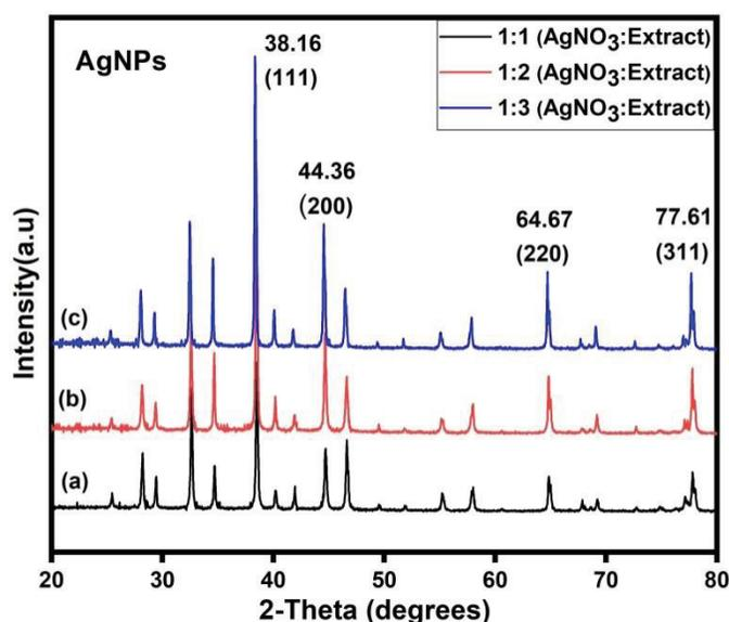
**FIGURE 3.** XRD of biosynthesized AgNPs from AgNO<sub>3</sub> to *Laggers* plant extract ratio of (a). 1:1, (b). 1:2, and (c). 1:3
