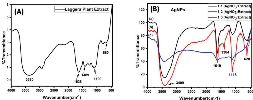
**FIGURE 2.** FTIR Spectra of (A). *Laggers* plant extract (B). biosynthesized AgNPs from AgNO<sub>3</sub> to plant extract ratio of (a). 1:1, (b).1:2, and (c).1:3
