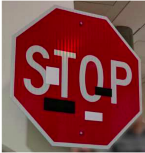
Figure 1.2: State of the art computer vision systems for self-driving cars think this stop sign is actually a 45 km/h speed limit sign. This confusion is caused by the black and white stickers applied to the sign. Without them, the stop sign is correctly identified. Image taken from Eykholt et al. [2018].
