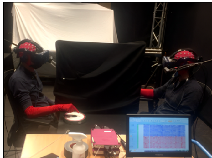
Figure 6-2: Snapshot taken during data collection showing two participants wearing HMDs and matching gloves, a separating screen, the video cameras, and EEG system
