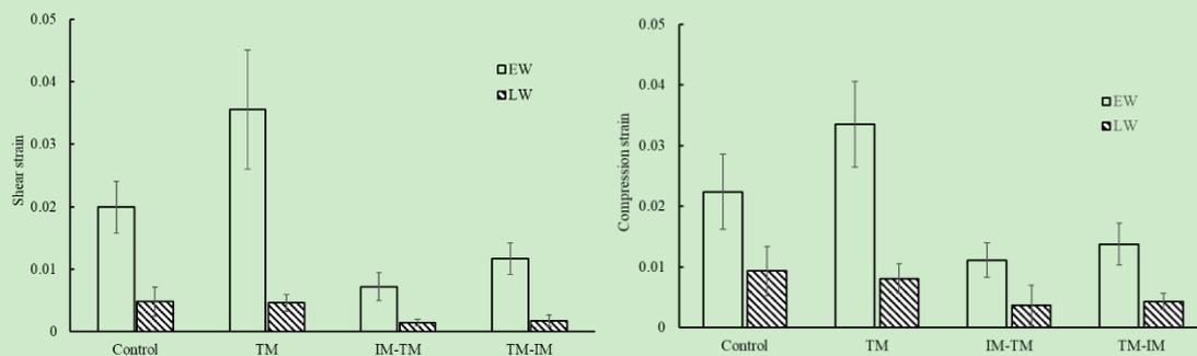
Fig.8 Shear strain distribution in earlywood (EW) and latewood (LW) of the four different types of specimens at compressive stress 4.8MPa
