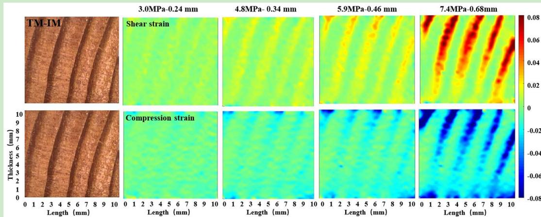
Fig.7 Shear strain (top row) and compression strain (bottom row) of four different types of specimens at four different compressive stress and displacement steps
