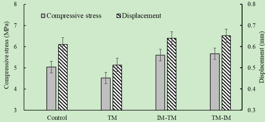
Fig.2 Compressive stress and deformation of four different types of specimens
