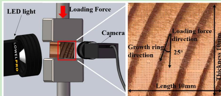
Fig.1 Illustration of the compression and DIC test set-up
