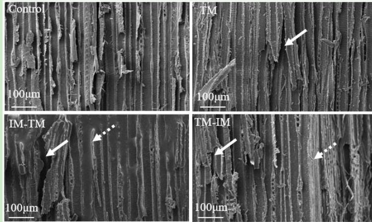
Fig.6 Ruptured tangential section microstructure of four different types of specimens. Solid arrows indicate the rupture of wood fiber. Dashed arrows indicate the accumulation of resin
