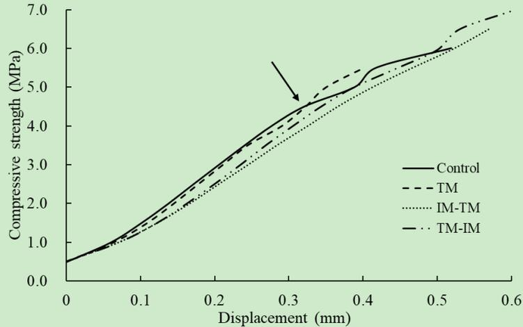
Fig.3 Relationship between compressive stress and deformation of four different types of specimens. Arrow indicates an inflection point divided the curve into two domains
