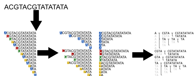
FIGURE 9 A suffix tree is a data structure containing all the possible suffixes in a chain of characters. Namely, suffixes that share the same prefix are considered to be part of the same branch, diverging into separate branches when the prefixes no longer match.
