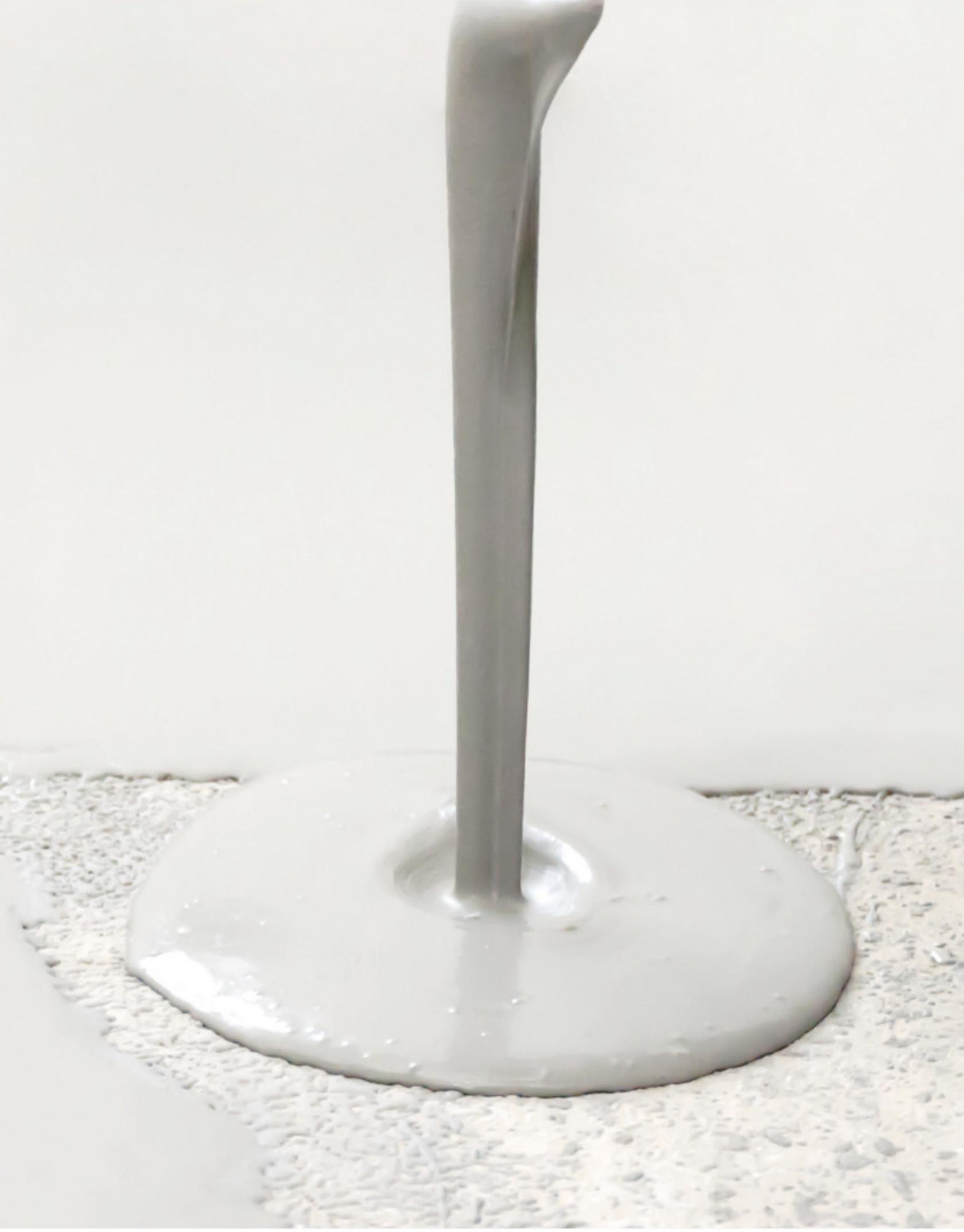
Low-carbon and sustainable alkali-activated cement in the flow state.
