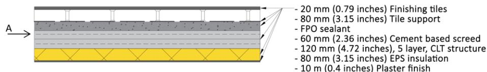
**Figure 2** Cross-section of the CLT balcony floor with and overview of applied materials.
