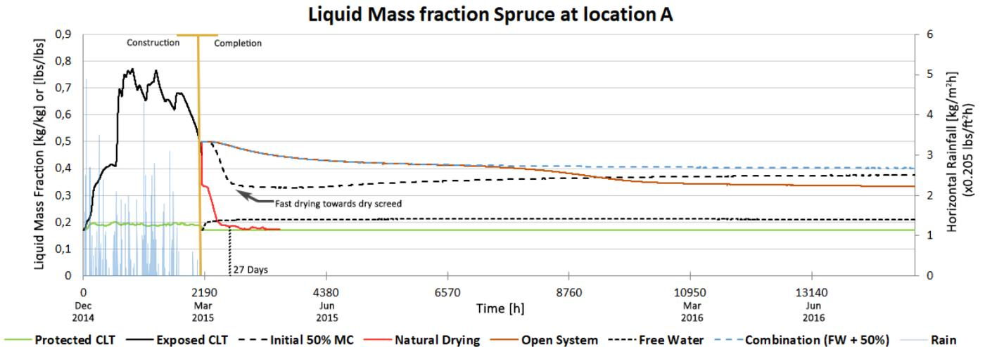
**Figure 4** Summary of the absolute Liquid mass fraction [kg/kg] or [lbs/lbs] in the location A (left) for different solutions and approaches compared with the current degraded state.
