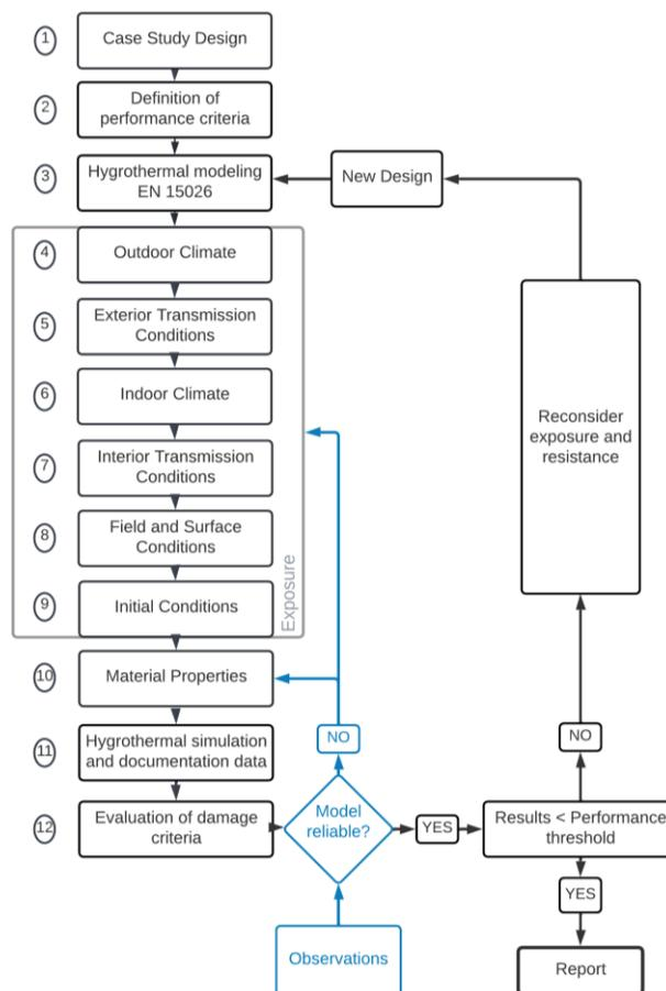
**Figure 1** Methodological framework as a guideline to perform performance assessment by means of HAM-simulations
