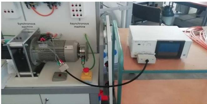
Fig. 2. Measurement setup using Hioki IM3536 and L2000 probes.
