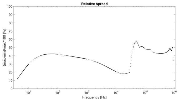
Fig. 4. Data spread of the individual motors plotted in Fig. 3, for each frequency the difference between highest and lowest value is compared to the highest one.
