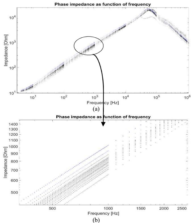
Fig. 3. (a) Variation of impedance by (a) full frequency range for 750W induction machines and (b) focusing around 1kHz frequency. Motor number eight shown in blue is of a different batch.
