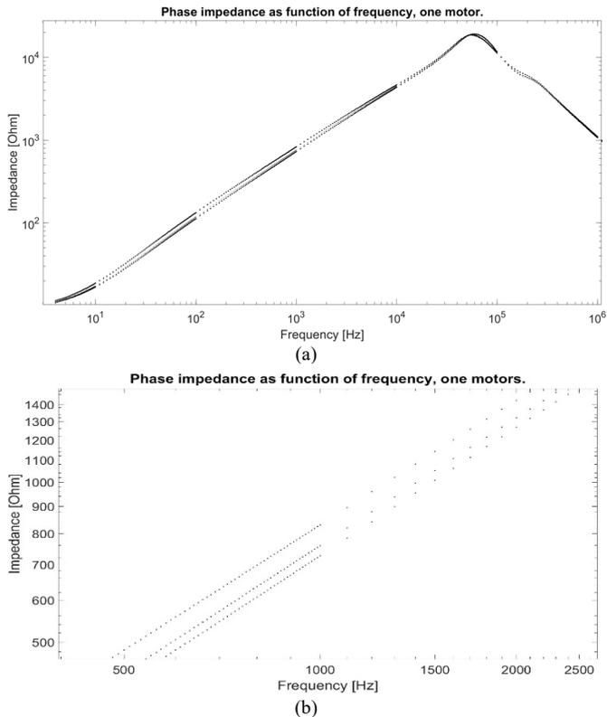
Fig. 5. Impedance of the 3 phases of an induction motor plotted together, a difference can be observed albeit smaller than in Fig. 3: (a) full frequency range and (b) focusing around 1 kHz frequency.
