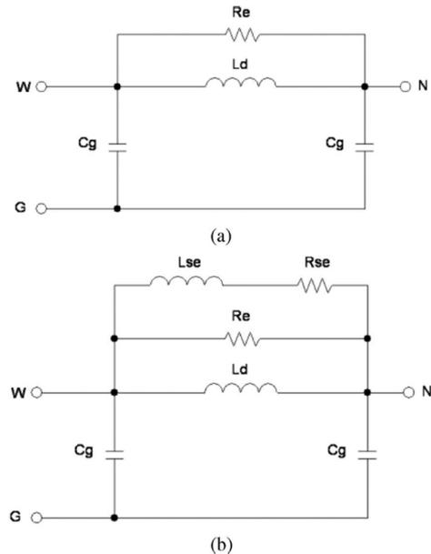
Fig. 7. HF motor winding model as presented by [3], (a) without skin-effect and (b) with skin-effect modelled.
