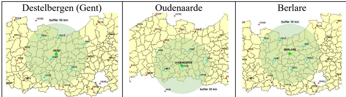
Figure 1: Location of the survey sites in green; location of the 6 nearest CORS within a maximum distance of 30 km; red location of the other CORS
