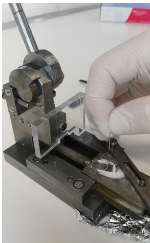
Figure III.1 Custom-made tableting machine used to compress the OCORS-0.5mm blend.
